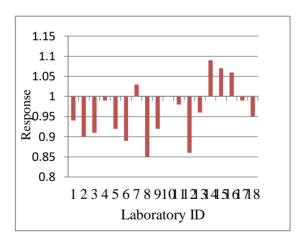
**Figure 2:** *Response factor of known dose* for *Cs-137 with 0 degree incidence angle*
