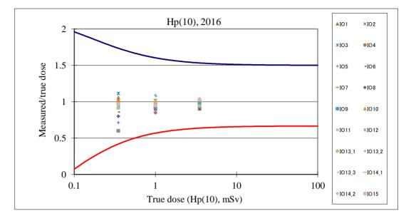
**Figure 4:** The trumpet curve of response factor versus the true dose for Hp(10)
