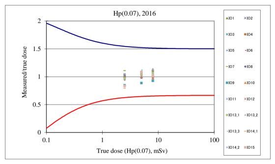
Figure 5: The trumpet curve of response factor versus the true dose for Hp(0.07)
