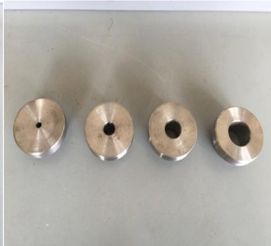
Fig 3: The collimators for radioisotope source at NEF of Dalat university
