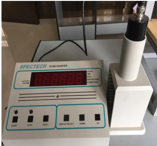
Fig 4: The gamma-ray detector at NEF of Dalat university
