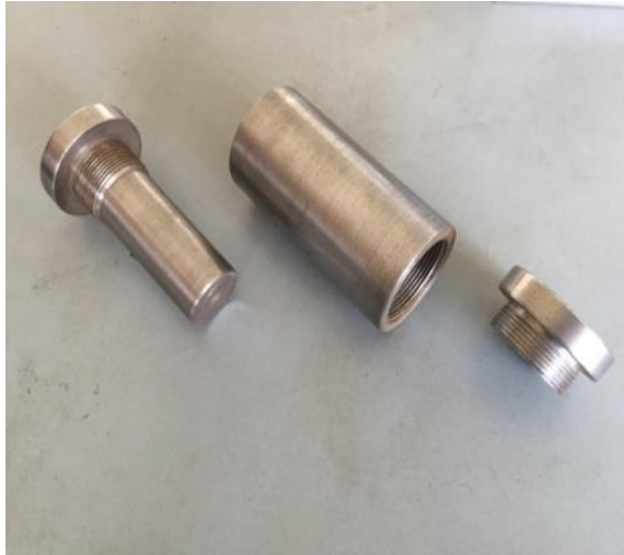
Fig 2: The radioisotope source box at NEF of Dalat university
